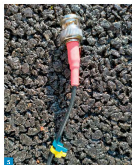
Fig. 5: Some feeders. Notice how the colour-coded one with cable ties is clearly recognisable.
